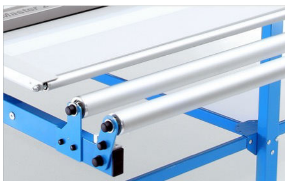
Upper version of a fabric feeder makes it easier to unroll the material
